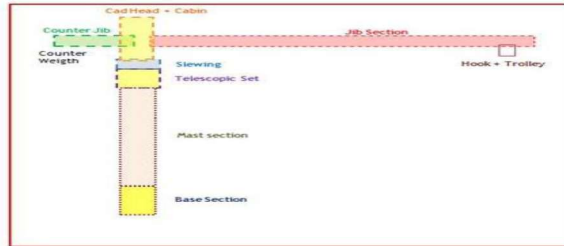
Gambar 2. 5 Struktur Crane Hydraulic Slewing
