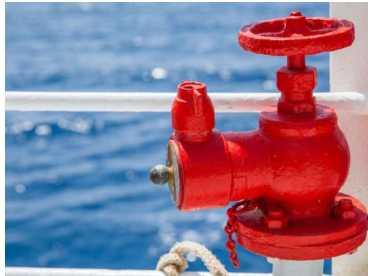
Gambar 2.12 : Fire Hose System
