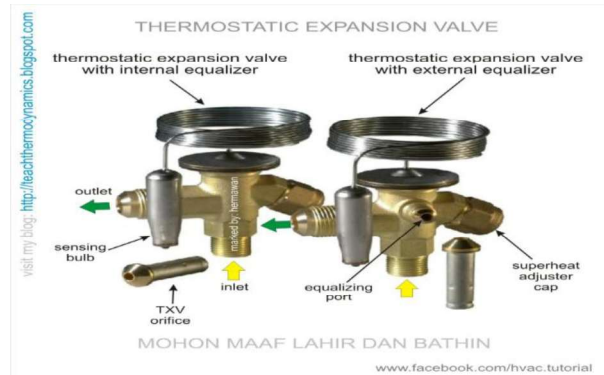
Gambar 2. 19 Katup expansion
