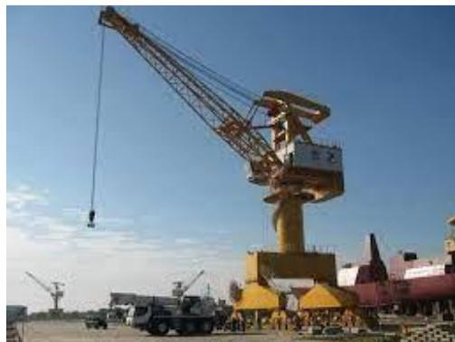
Gambar 2.8. *Level Luffing Crane*
