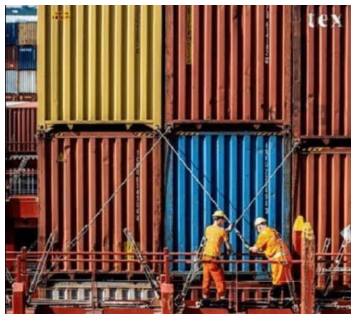
Gambar 2.2 Pengikatan/ lashing single lashing pada peti kemas Sumber : https://www.researchgate.net/figure/Lashing-and-de-lashing-in-Antwerp-port-photo-courtesy-of-Cepa_fig1_344015474
