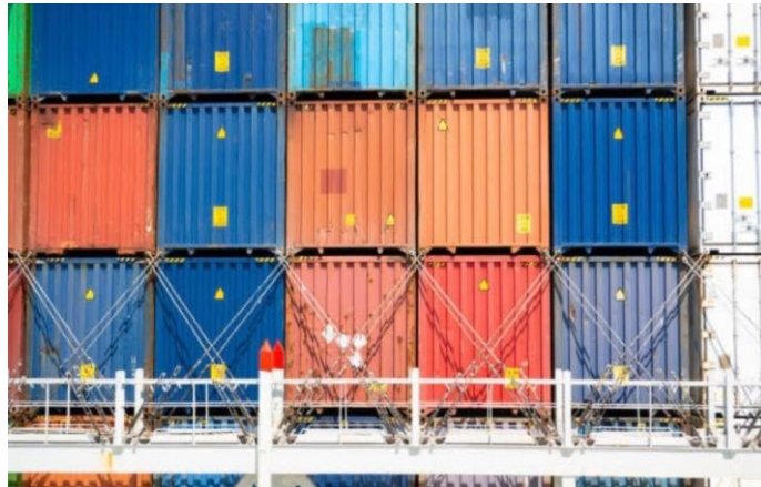
Gambar 2.3 Pengikatan/ lashing double lashing pada peti kemas. Sumber : https://www.shutterstock.com/id/image-photo/different-color-white-reefer-containers-loaded-2324679477
