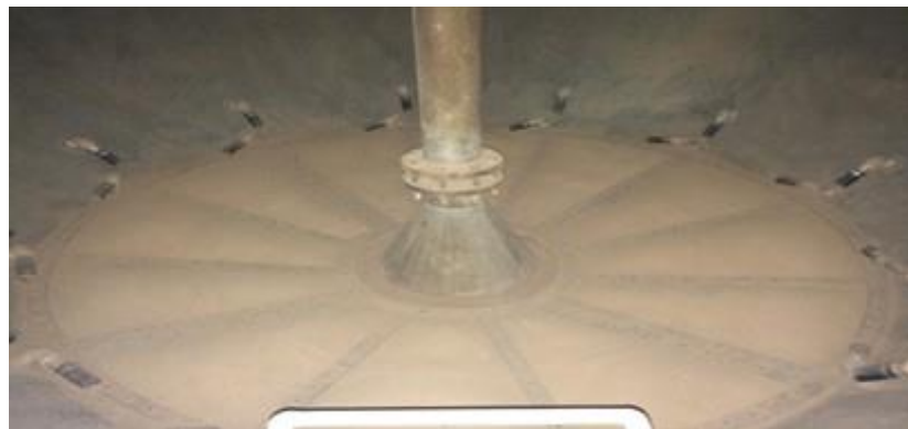
Gambar 2. 7 Slide Canvas Didalam Tangki Dry Bulk (Barite) Sumber : repository.pip-semarang.ac.id
