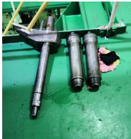
Gambar 2.5 Fuel Oil Injection Valve Sumber : MV. Hanglima
