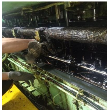
Gambar 4. 5 Proses Bongkar Fuel Injection Pump Sumber : Dokumen Penelitian (2023)
