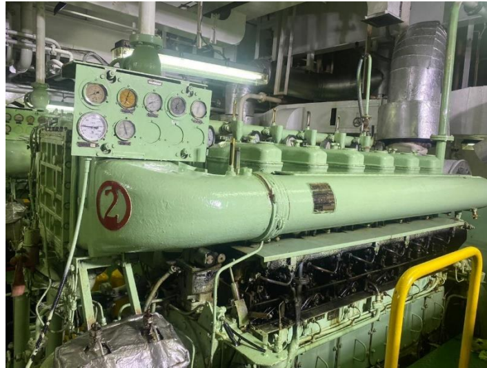
Gambar 4. 2 Mesin Diesel Generator MV. Tanto Express Sumber : Dokumen Penelitian (2022)
