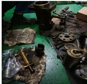
Gambar 4. 4 Bongkar Fuel Injection Pump Sumber : Dokumen Penelitian (2023)
