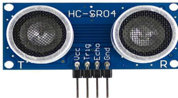
Gambar 2.5 Sensor Ultrasonik
