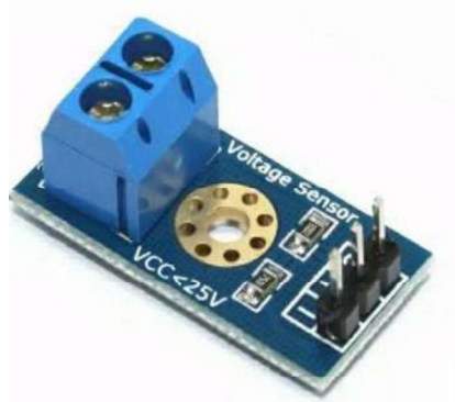
Gambar. 2.14. Voltage Sensor Divider
