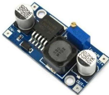
Gambar. 2.12. Step Down Converter LM2596
