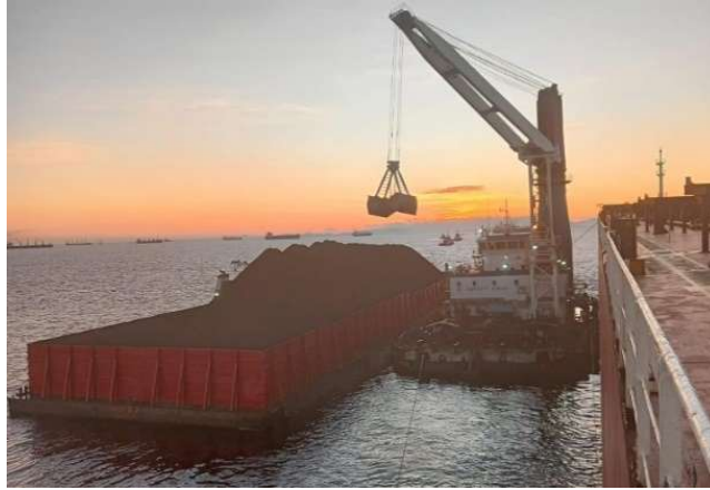
Gambar 2. 2 Proses Ship to ship Penyandaran Tonkang ke Floating Crane Sumber: Dokumen Pribadi
