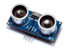
**Gambar 2.12** Sensor ultrasonik HC-SR04 Sumber: https://www.e-gizmo.net/
