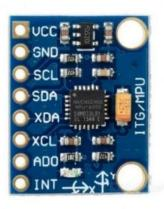
**Gambar 2.15** Sensor *gyroscope* MPU 6050 Sumber: https://www.elementzonline.com/
