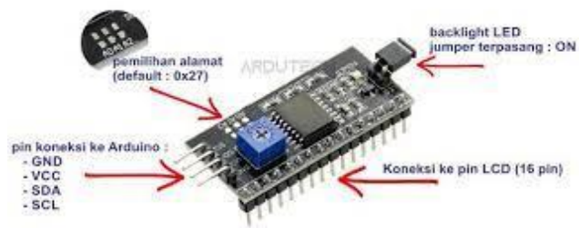
Gambar 2 . 13 Modul I2C ( Inter-Integrated Circuit )
