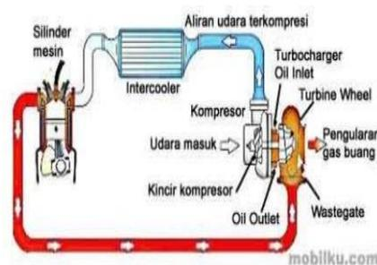
Gambar 2. 11 Sistem sirkulasi turbocharge
