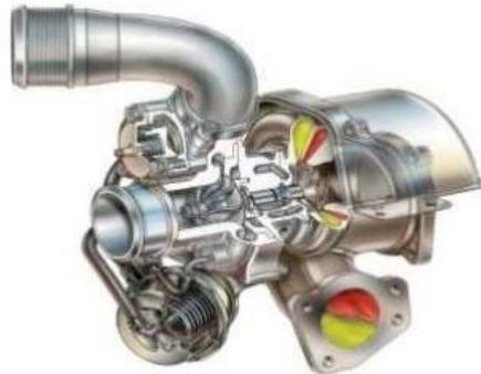
Gambar 2. 16 *Variabel scrol turbocharge*
