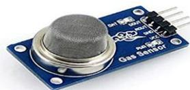
Gambar 2.4 *Smoke detector* ( $MQ_2$ )
