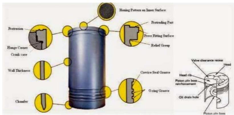
Gambar 2.6. *Silinder liner*
