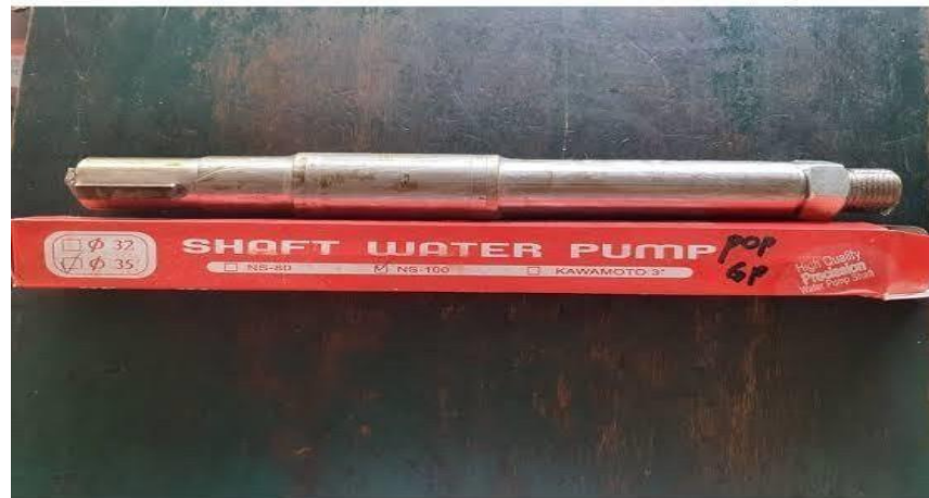
Gambar 2. 10 Shaft water pump
