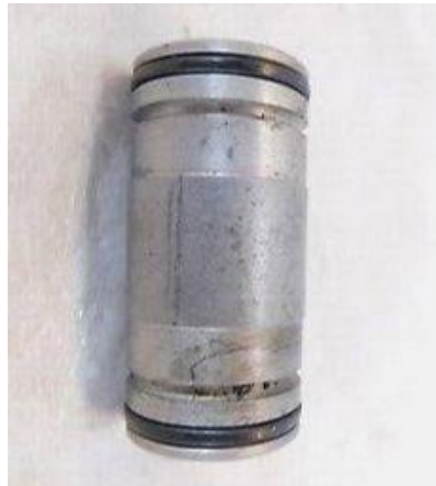
Gambar 2. 17 Cooling Water Inlet Joint
