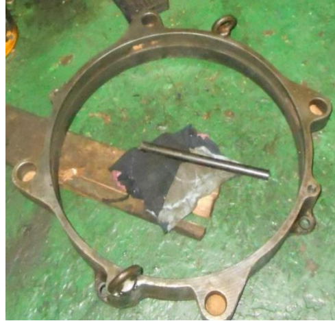
Gambar 2. 15 Water Guide Jacket
