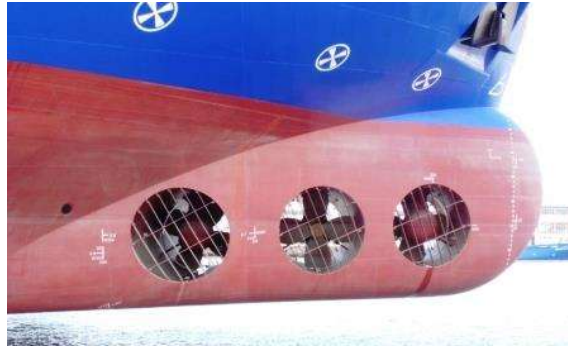
Gambar 2. 8 Bow Thruster on AHTS Vessel
