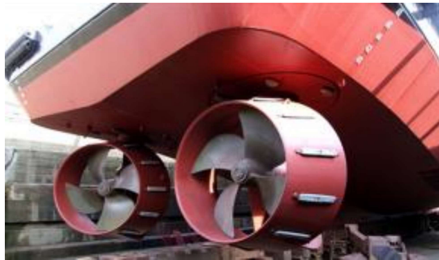
Gambar 2. 7 Twin Propeller with Azimuth Thruster
