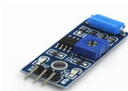
Gambar 2. 2 Sensor Sw-420 (Sumber: mectronica.com.co)
