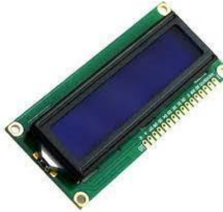
Gambar 2. 6 Liquid Cristal Display (LCD)
