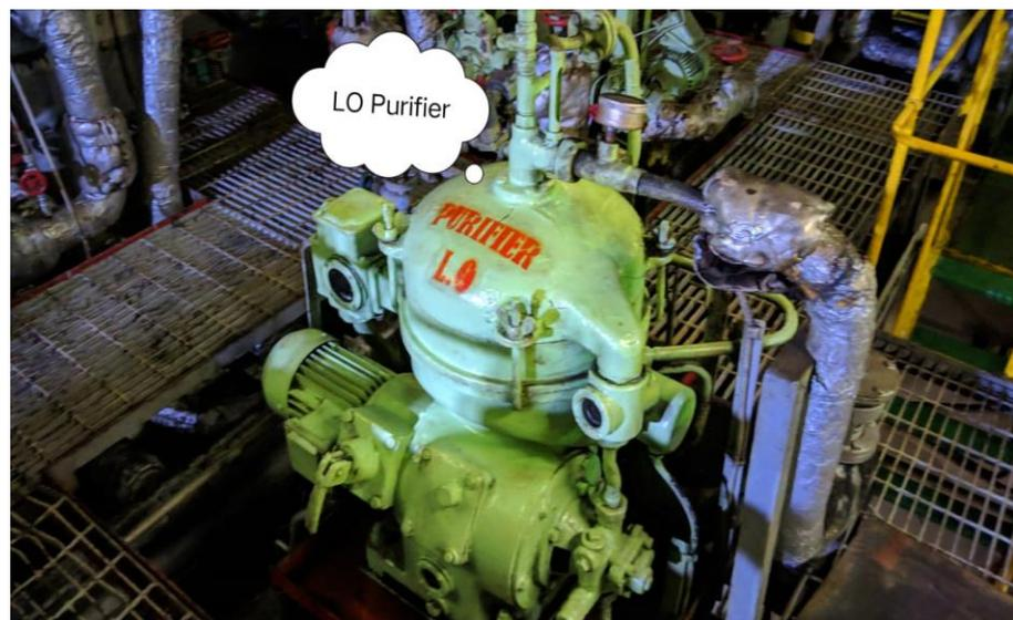
Gambar 2.5 *Lubricating Oil Purifier*
