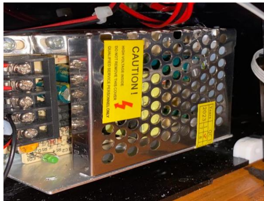
Gambar 2. 4 Power supply AC 220V to DC 12V (Sumber: Dokumen pribadi)
