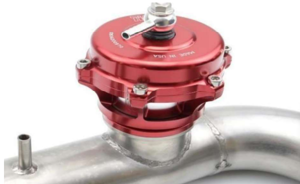
Gambar 2. 8 Blow Off Valves
