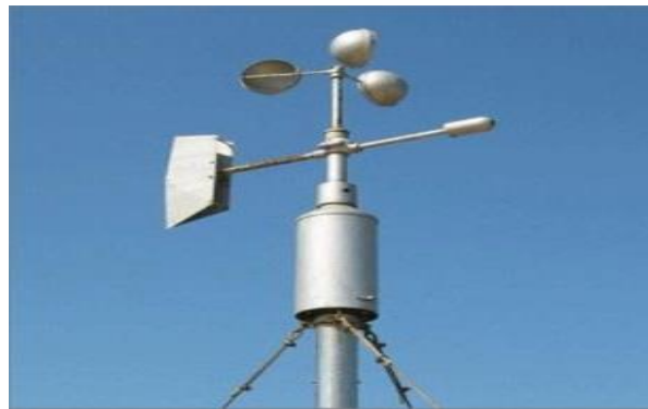
Gambar 2.1. Cup Anemometer Sumber: Pangetsu (2014)
