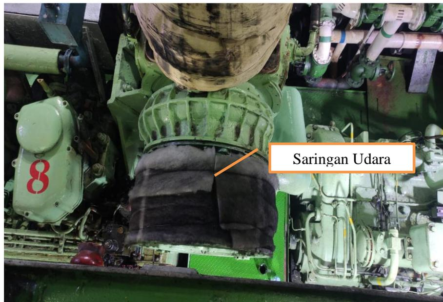
**Gambar 2. 7 Turbocharge**
