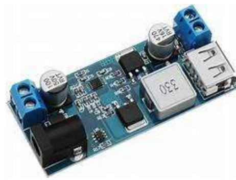
Gambar 2. 13. Transformer Step-Down 12vdc – 5vdc
