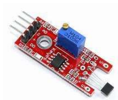
Gambar 2. 14. Sensor RPM ( Hall-Effect Sensor )
