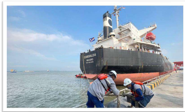
Gambar 2.2. Pemasangan After Spring Line ke Bolder saat Proses Clearance In
