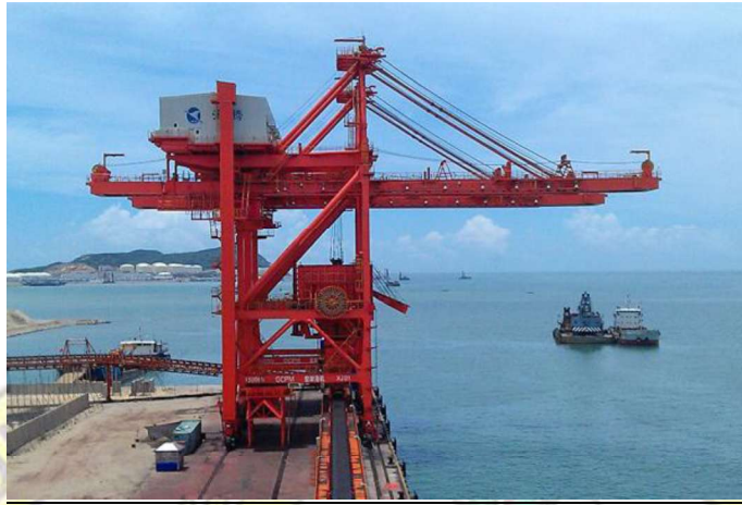
Gambar 2. 17 Shore-based grab crane
