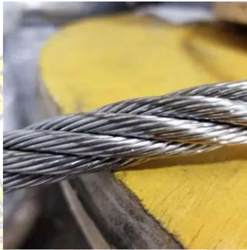
Gambar 2. 5 Bright Wire Rope
