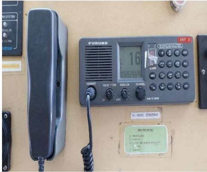
Gambar 2. 8 VHF ( Very High Frequency ) Radio Telephony Sumber: Data Peneliti (2023)
