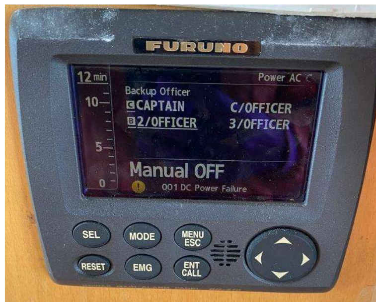
Gambar 2. 1 Bridge Navigational Watch Alarm System Sumber: Data Peneliti (2023)
