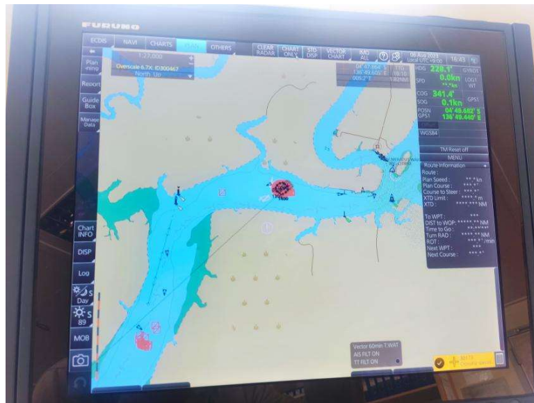
Gambar 2. 5 Electronic Chart Display and Information System Sumber: Data Peneliti (2023)
