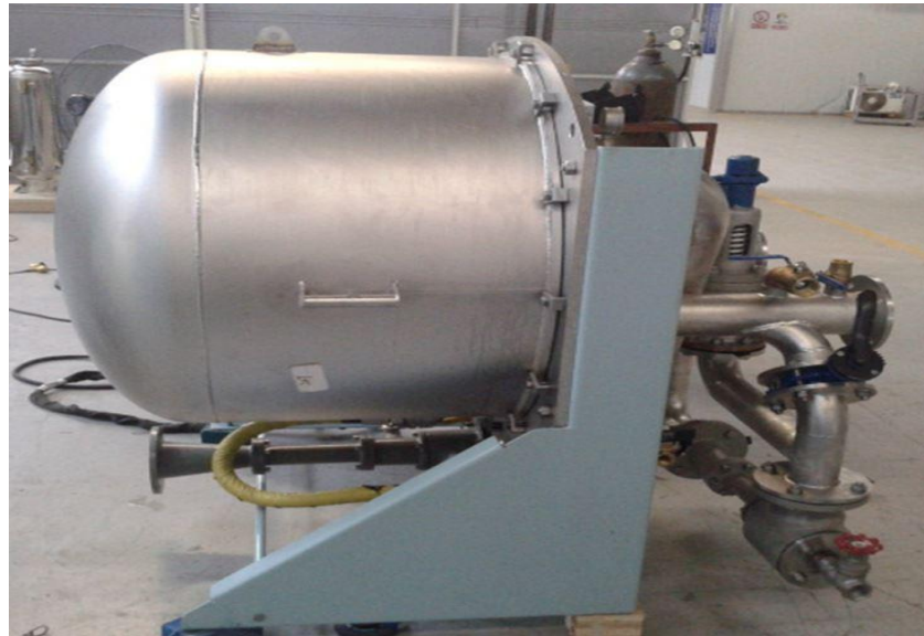
Gambar 2.1 Fresh Water Generator
