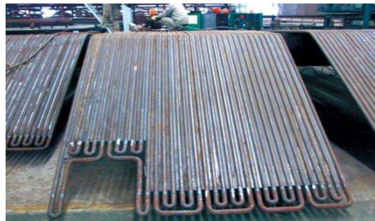
Gambar 2. 7 Water Wall Tube Boiler
