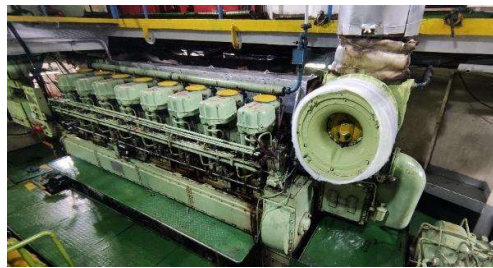
Gambar 2. 17 Single-Turbocharger Sumber: Dokumentasi penelitian
