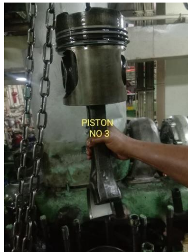
Gambar 4. 4 Piston No.3 Diesel Generator dicabut Sumber : Dokumen Peneliti (2023)
