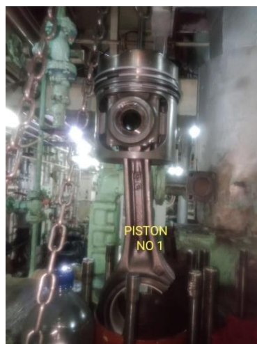
Gambar 4. 5 Piston No.1 Diesel Generator dicabut Sumber : Dokumen Peneliti (2023)
