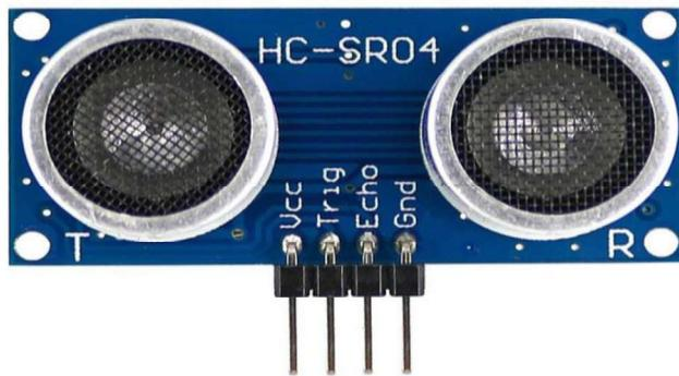
Gambar 2.5 Sensor Ultrasonik
