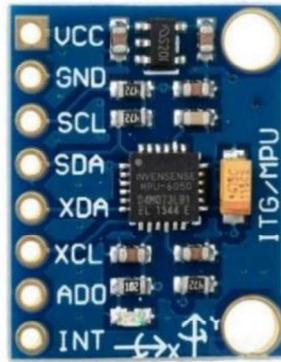
**Gambar 2.15** Sensor *gyroscope* MPU 6050
