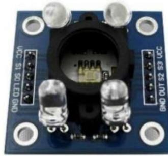
**Gambar 2.14** Sensor warna TCS 3200
