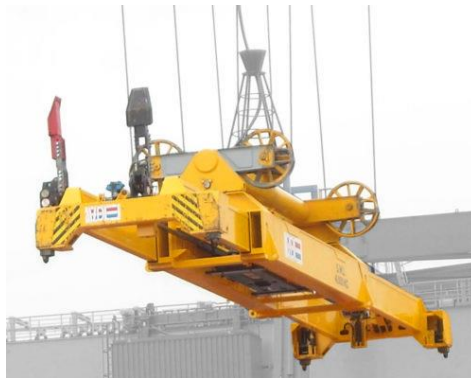
Gambar 2. 1 Spreader (Sumber: www.greenfieldpi.com )
