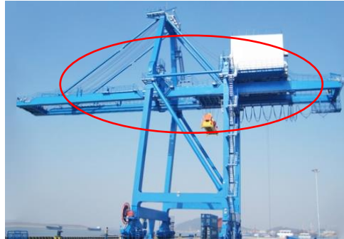
Gambar 2. 2 Boom (Sumber: www.hycranes.com )
