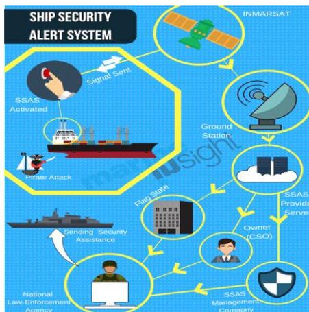
Gambar 2.3 Sistem kerja *Ship Security Alert System (SSAS)*
