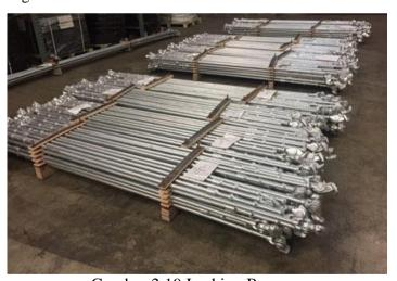
Gambar 2.19 Lashing Bar Sumber: <a href="https://www.pacificmarine.net">https://www.pacificmarine.net</a>
