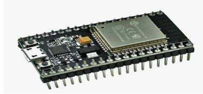
Gambar 2.1 Node MCU ESP32S
