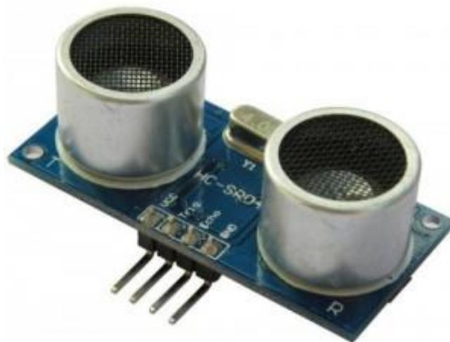
Gambar 2. 1 Sensor *Ultrasonik*
