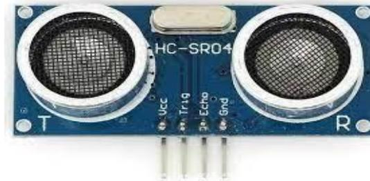
**Gambar 3. 2 Sensor Ultrasonik**
