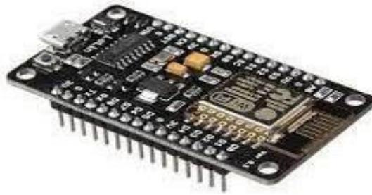
**Gambar 2. 1 NodeMCU ESP**
