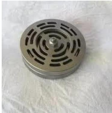
Gambar 2.6 *Low Pressure Delivery Valve*
