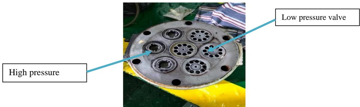
Gambar 2.4 valve high & low pressure
