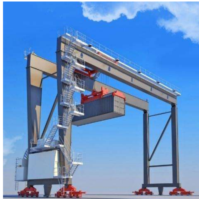
Gambar 2. 1 Rubber Tyred Gantry Crane (RTG)
